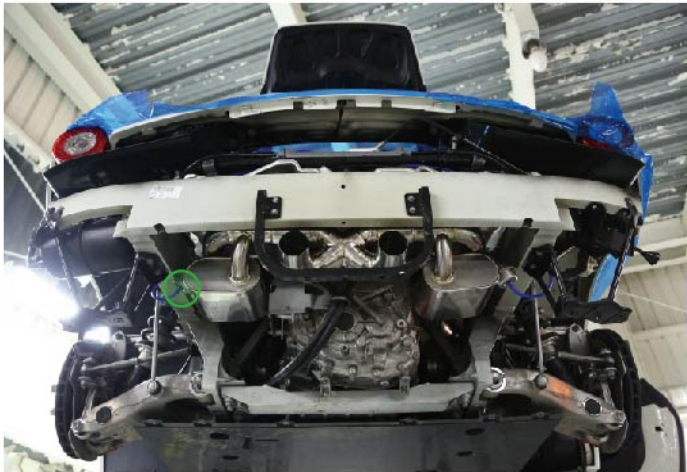
► Please adjust left muffler and make sure valve wont collide with car body As long as the muffler is not touching the car body is within normal range
